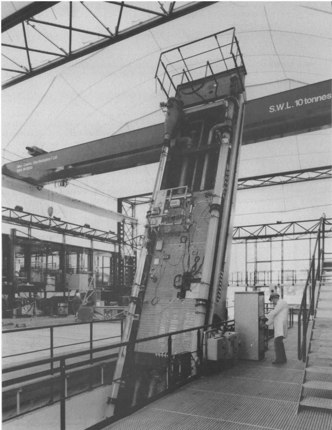
Figure 1. Photograph of the multiphase flow test facility at SCR, the mud loop is shown in the right-hand side with the three-phase loop on the left.
